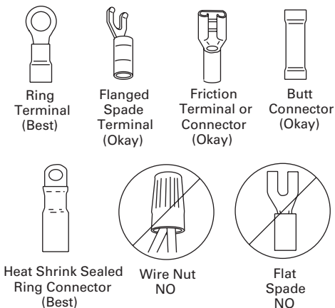
FIGURE 9-16: Cable Terminals and Connectors
